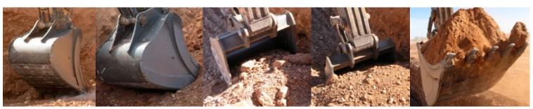
The Volvo bucket makes penetration, then is pulled into the material and fills smoothly. After filling, the bucket cradles the material and is ready for dumping.
