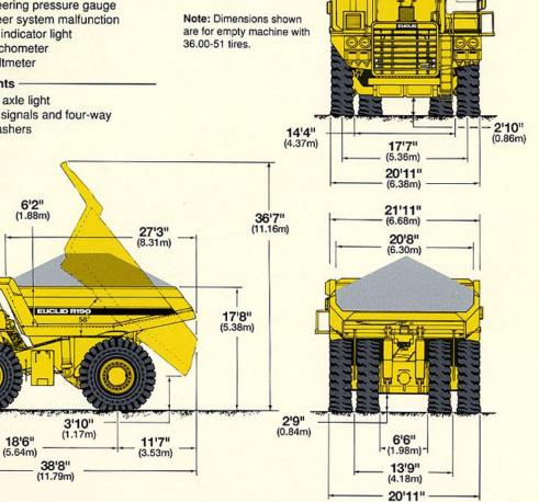
The Euclid Field Heap illustrated in the side view above maintains a 2:1 heap ratio from the floor/tail chute junction to the peak of the load profile. The SAE 2:1 heap ratio is actually a 1:1 heap ratio from floor/tail junction to the top body edge, then switches to a 2:1 heap ratio to the load peak. The Euclid Field Heap is more representative of field loading practices and payload distribution. Euclid body capacity ratings are based on the field heap philosophy.
