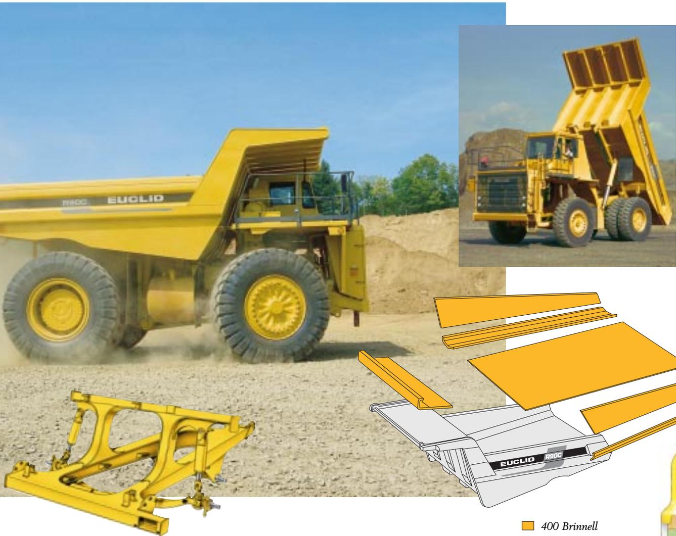
All Euclid hauler bodies are continuously exhaust-heated regardless of body position. The body is designed to maintain load integrity, effectively shed material during the dump cycle, and isolate exhaust from the cab and air filters.
