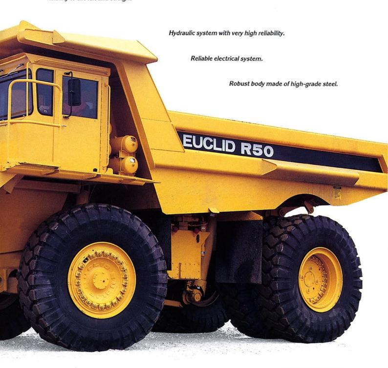
Rugged frame built to take heavy stresses over a long period of time. Frame junctions with large radii between all sections eliminate all direct stress concentrations. Reliable dual-circuit brake system with high availability. Nitrogen/oil suspension struts all around for good comfort and mobility, even on poor surfaces. The suspension characteristic can be adapted to the actual conditions on the worksite.
