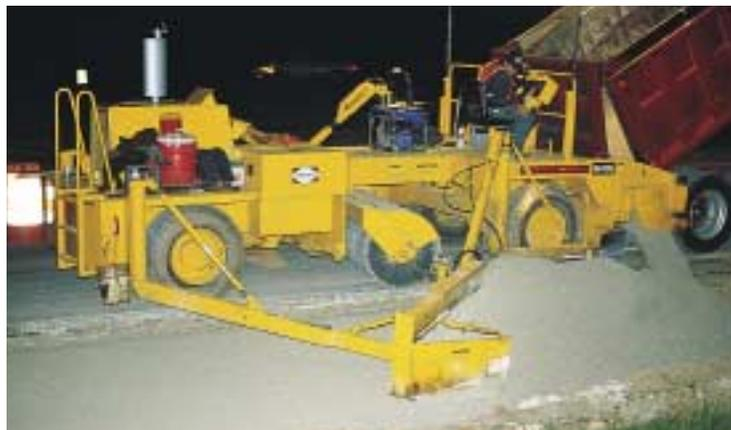
**Truck Hitch:** Two bearing equipped push rollers mounted on an oscillating frame with electric/hydraulic actuated, roller equipped clamp arms; quickly grips and secures a truck in proper attitude for unloading material into the machine's hopper; automatically compensates for both minor lateral and directional misalignment of truck with road widener with no exposed secondary slide mechanisms.
