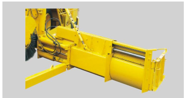
**3' (914 mm) Hydraulic Strike-Off Extensions:** A hydraulically extendible strike-off extension (left side or right side) that can be mounted on the outer end of either the standard 3' (914 mm) or 6' (1829 mm) contoured strike-off sections to provide additional "on-the-go" variable operating width flexibility in conjunction with the standard 2' to 3' (610 mm-914 mm) telescoping sections.
