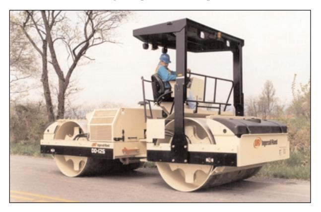
The DD-125 features dual 84 inch (2135 mm) wide drums with 2500 vpm (41.7 Hz) frequency for high performance capability on main line highway and other large paving jobs. Operating weight of 14 tons (12.7 metric tonnes) meets all state D.O.T. static rolling requirements. The DD-125 has a nominal capacity to more than 300 tons (265 metric tonnes) of HMA per hour.
