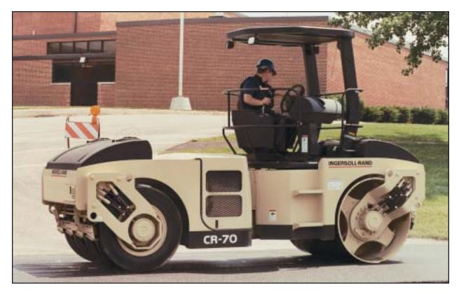
The CR-70 is a 6.5 ton (6 tonnes) weight unit that utilizes the forces of vibration and tire manipulation to achieve required density and smoothness on Hot Mix Asphalt (HMA) pavements. The unit can also be used to compact granular or mixed soils, crushed aggregates and cement-treated bases.
