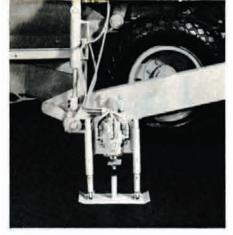
Only ten minutes required to switch attachment to opposite screed arm. Extensions are available to match screed widths up to 16 feet.
