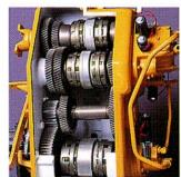
The exclusive **Champion 8400** grader transmission is now in service in more than 10,000 units. Evenly proportioned gear ratios provide precise, job-matched speeds for any grading application. A new "Smart Shift" feature lets the operator easily customize shift patterns to the job at hand.
