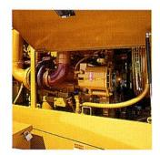
Job-matched dependable Cummins diesel power offers superior fuel efficiency as the engine's peak torque is matched to transmission shift points. Optional side panels are lockable and provide easy access for routine maintenance.
