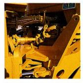
Twin 5 inch diameter hydraulic cylinders articulate the frame 22°. The main hinge pins are 3" in diameter and are contained within sealed housings. Anti-drift lock valves ensure drift-free operation.
