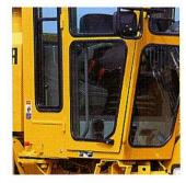
Series IV cab changes include a 'sweep-out' cab floor, easy-to-use door releases and re-enforced door and window frames. Twopiece door glass design makes glass replacement easier and less costly than ever before!
