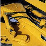
Patented dual-cylinder circle drive uses direct-acting hydraulics for exceptional turning and holding power under full load. Circle drive system is protected against impact damage by an overload cushion valve as standard equipment.
