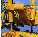
Rugged design of the standard fixed-point blade lift system provides fewer moving components for low maintenance.
