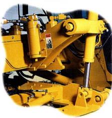
The heavy-duty 2 1/2" piston rods provide maximum strength to Series IV blade lift cylinders for tough applications like mining and forestry. Standard equipment includes nitrogen precharged piston accumulators to absorb impact loads; isolation valves ensure rocksteady blade control in fine grade applications where shock protection is not needed.
