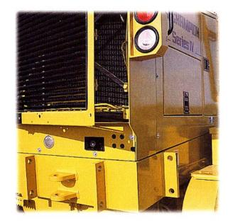
Series IV is built on a solid foundation of already proven Champion features. Some of these include: the rear perimeter frame, the first user lifetime frame warranty and a hinged rear grill for easy radiator cleaning.
