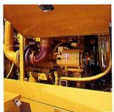
Job-matched dependable Cummins diesel power offers superior fuel efficiency as the engine's peak torque is matched to transmission shift points. Optional side panels are lockable and provide easy access for routine maintenance.
