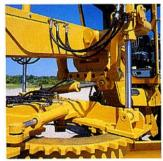
Lift system provides widest lift cylinder stance of any grader for maximum stability and reduced end-to-end blade interaction, resulting in better fine grade control.
