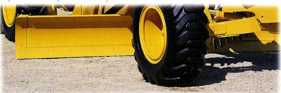
With its 72° front axle steering angle, Series IV moves comfortably in confined work areas. The tight turning radius means faster finishing in cul--de-sacs and less following-up in the corners.
