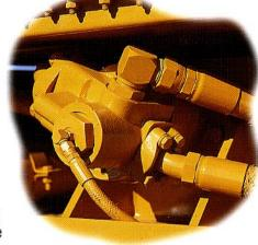
Foot-pedal operated full-oil clutch provides superior "inching" capability and precise control in tight working
