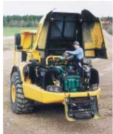
*Access to the whole engine compartment is superb thanks to the new engine hood. An access ladder incorporated in the front grille makes it very easy to reach the various service points.*
