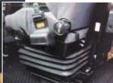
*An air suspension operator's seat improves comfort.*
