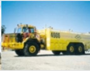
*A service vehicle based on the A35C for hauling fuel, cooling agents and lubricants to large dump trucks over 130 tonnes. Thanks to its off-road performance it can reach the trucks wherever they happen to be in the huge open cast mine in Hunter Valley, New South Wales, Australia.*
