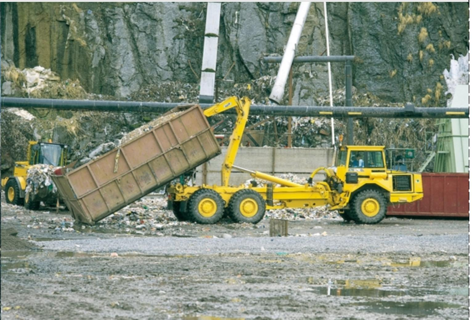
*An A25C Hook Lift at a recycling facility in Vaasa, Finland. With the interchangeable loading system the same vehicle can be used for many different jobs.*
