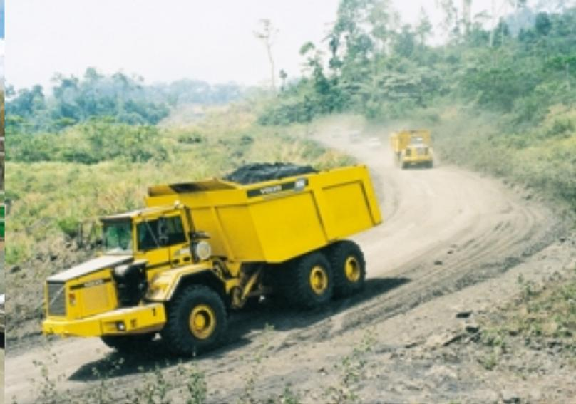
*In Sumatra, Indonesia, an A35C Coal Hauler is used by the operator P.T.Bukit Sumur to haul coal. The body is specially built for low-density materials and holds all of 36 cubic metres.*
