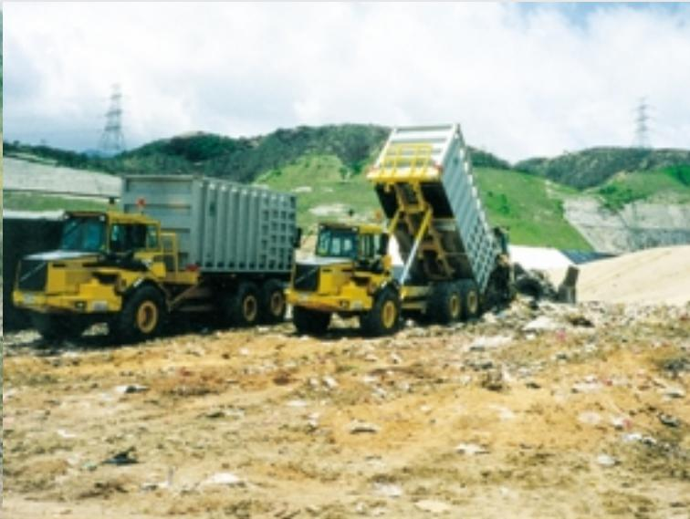
*Two out of the ten A25C Container Haulers that handle waste in Hong Kong. Thanks to their low ground pressure they can move anywhere on the dump with safety.*
