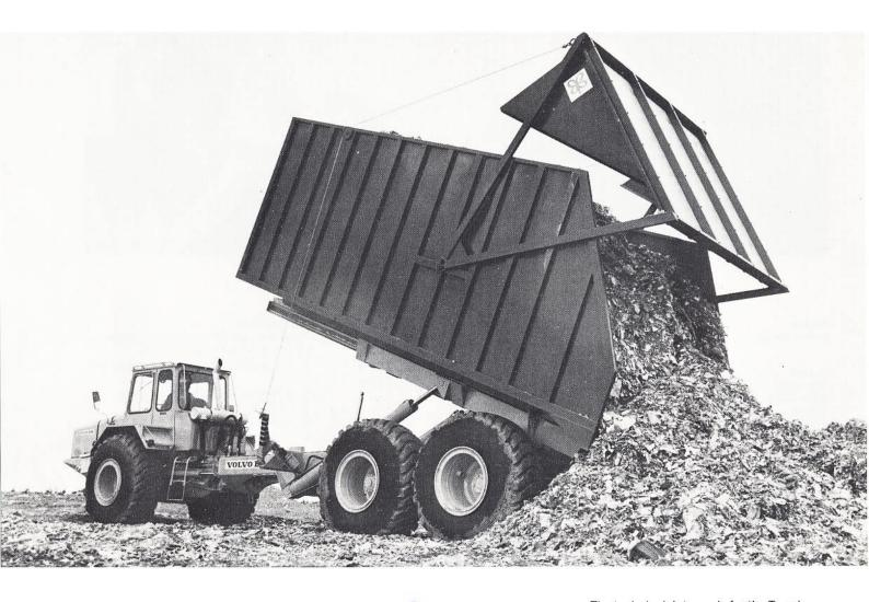
The Volvo BM 861 TC is designed for hauling refuse at tips, and from loading station to tip.
