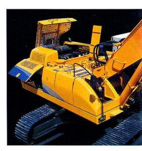
• Easy Access Oil Filter - The engine oil filter is conveniently located for easy access to inspect or change.
