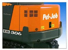
Because some knocks are unfortunately unavoidable, the wrap-around counter-weight protects the rear of the machine. The steel cover is mounted recessed in relation to the counterweight to improve its protection.
