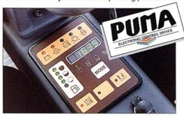
The PUMA system on the EB 306 continuously monitors all the machine's vital functions and immediately informs the operator if there is a fault. The operator is therefore free to concentrate fully on operating the machine.
