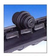
Ride comfort is considerably improved thanks to the profile of the tracks and the alternating position of the guides which provides permanent contact with the rollers.
