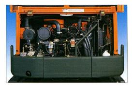
The wide soundproofed cover opens completely, giving excellent accessibility to the engine: all the maintenance and checking points are close at hand to save time. The steel cover is mounted recessed in relation to the counterweight to improve its protection.
