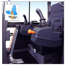
Operator comfort is a priority for Pel-Job. The operator's cab is spacious and easily accessible. The hydraulic controls are power-assisted and very progressive for more flexibility and precision. Pel-Job's new ergonomic manipulators feel good and are complemented by side arm rests which give a natural and very comfortable operating position.
