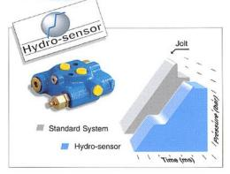
The hydrosensor valve (Pel-Job patent) on the slewing circuit damps the pressure peaks and hydraulic shocks common on starting and stopping on conventional circuits. The result: a progressive pressure increase, greater flexibility and precision and less stressed and therefore more reliable mechanical parts
