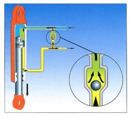
The dipper ram is equipped with an automatic energy recovery system which recycles the hydraulic oil displaced from the ram and speeds up the arm lowering movements.
