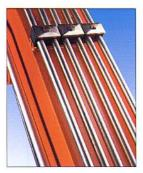
Very effective corrosion protection: all the nuts and bolts, the pins and the hydraulic pipes are zinc-plated and passivated.
