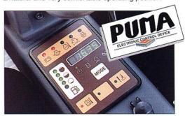
The PUMA system on the EB 25.4 continuously monitors all the machine's vital functions and immediately informs the operator if there is a fault. The operator is therefore free to concentrate fully on operating the machine.
