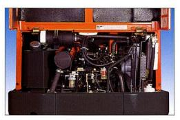
The wide soundproofed cover opens completely, giving excellent accessibility to the engine: all the maintenance and checking points are close at hand to save time. The steel cover is mounted recessed in relation to the counterweight to improve its protection.
