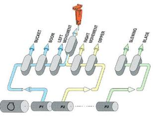
Three pumps each supply a separate hydraulic circuit in order to ensure total independence of each movement. Thus, for example, turret slewing or blade lifting are completely independent of all the equipment or travel movements.
