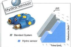
The hydrosensor valve (Pel-Job patent) on the slewing circuit damps the pressure peaks and hydraulic shocks common on starting and stopping on conventional circuits. The result: a progressive pressure increase, greater flexibility and precision and less stressed and therefore more reliable mechanical parts
