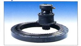
A Pel-Job exclusive: the radial piston slow slewing motor. This motor has a very high torque for flexible manoeuvres, and drives the crown directly without a mechanical reducer. The result is fewer moving parts and therefore less risk of wear. The automatic hydraulic brake integrated in the slewing motor immobilises the turret in all positions and guarantees optimum working safety even on a slope.
