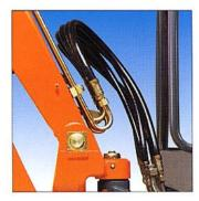
The hoses which supply the equipment are mounted loose at the bottom of the boom. They suffer less friction and wear, and can be replaced, if necessary, very quickly.
