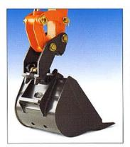
The exclusive Pel-Job quick hitch system, available as an option, makes it possible to change attachments very quickly.
