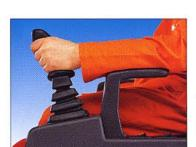
The ergonomically-designed Pel-Job armrests are placed in the immediate vicinity of the manipulators to support the wrists and forearms. The result : a perfect operating position, more precision and less fatigue.
