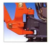
The boom is mounted on a double-swivel articulated pivot which enables a long pin to be mounted and provides greater rigidity in the boom-chassis link.
