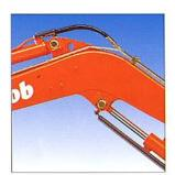
Computer-designed and then validated by resistance and endurance tests, the new boom concept is extremely sturdy thanks to the positioning of the welds in the low-stress zones.
