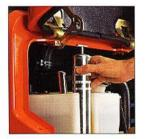
The diesel tank is made of transparent polyethylene so that the diesel level can be checked easily during filling. It also incorporates a very practical housing for the grease gun which is always to hand.
