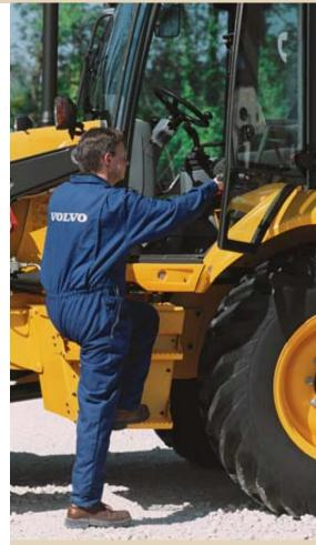
Handrails and three serrated steps for easy entry, exit.
