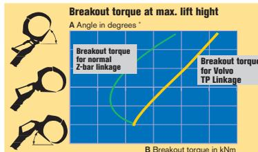
*The patented TP Linkage lift-arm system has superior breakout capacity throughout the lifting range and exceptionally good breakout force in the top position.*
