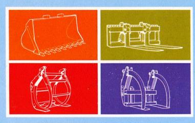
Volvo BM has always offered a wide range of attachments. Using the right attachment for the material or load to be handled boosts productivity and profitability. To achieve this we have equipped the Volvo BM 4400 with a wide variety of quality attachments, well-matched to the machine and their tasks. Also, the hydraulic attachment bracket makes it easy to switch attachments and jobs very quickly.
