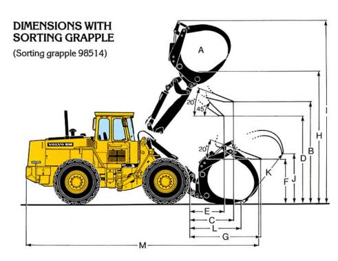
A = 1.4 m<sup>2</sup> (15 ft<sup>2</sup>) B = 3,575 mm (11' 9") C = 1,670 mm (5' 6") D = 3,140 mm (10' 4") E = 14300 mm (4' 8") F = 1,700 mm (5' 7") G = 2,440 mm (8') H = 4,310 mm (14' 2") I = 5,830 mm (19' 2") J = 2,700 mm (8' 10") K = 2,640 mm (8' 8") L = 1,680 mm (5' 6") M = 6,730 mm (22' 1")
