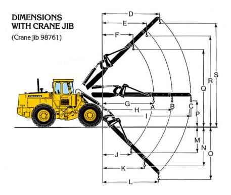
= 1,725 kg (3,800 lb) = 1,500 kg (3,305 lb) = 1,095 kg (2,415 lb) BODEF = 2,715 mm (8' 11") = 2,711 mm (6' 11") = 2,111 mm (6' 11") = 1,545 mm (5' 1") Ġ  $= 3,250 \,\mathrm{mm} \,(10'\,8'')$ = 3,250 mm (10'8') = 4,310 mm (14'2") = 5,440 mm (17'10") = 1,565 mm (5'2") = 2,200 mm (7'3") = 2,885 mm (9'6") = 1,910 mm (6'3") = 2,755 mm (9') Н K = 2,755 mm (9') = 3,660 mm (12') N OP 1,600 mm (5' 3") 5,255 mm (17' 3" Q =RS = 6,155 mm (20' 2") = 7,110 mm (23' 4")
