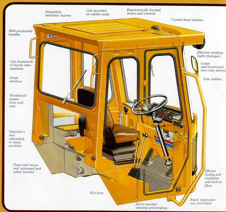
The cab is your workplace. You should be comfortable and be able to work safely and efficiently, regardless of the outside weather conditions. The Volvo cab on the 4200 is built to give you optimum comfort with easy-to-operate functions. The seat, levers, controls and instruments have been thoroughly tested and carefully planned and positioned.
