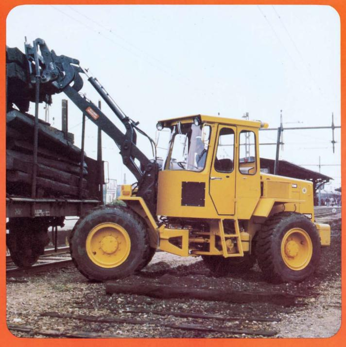
The Volvo 4200 has a well-designed loader unit with long reach, a smooth underside, parallel side-arm action and high side-arm attachment points. This means you can load wide vehicles from one side with short work cycles. Its precision and parallel side-arm action is ideal for handling fragile and palletized goods. The power-shift gearbox and articulated steering make it easy to position the load exactly where you want it.
