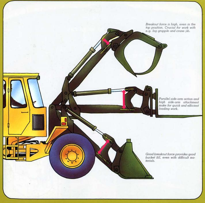
The loader unit is a crucial factor in determining the capacity of a loader. When widely varying tasks are performed, it is of the utmost importance that high performance be achieved at each task. The 4200 has a superb loader unit with the following advantages:
