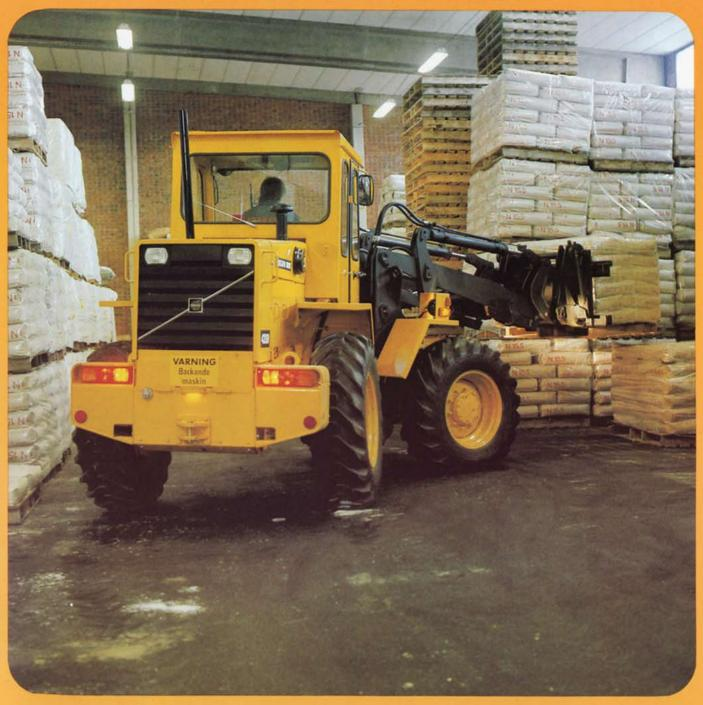
At stockyards, in warehouses and in harbours, the 4200 makes optimum use of available space. It's agility and manoeuvrability produces optimum efficiency. It is a compact machine giving you a good view to both front and rear. The 4200's good lifting height and generous reach enable you to work at high stacks. There is also a wide variety of attachments to choose from, each specially designed for efficient materials handling.
