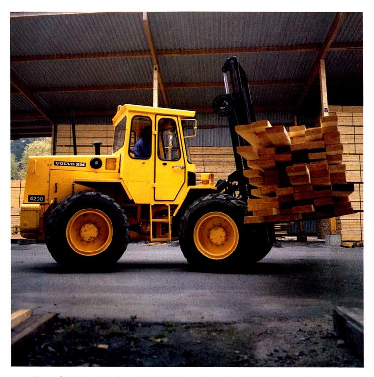
Specification Volvo BM 4200 equipped with fork carriage
