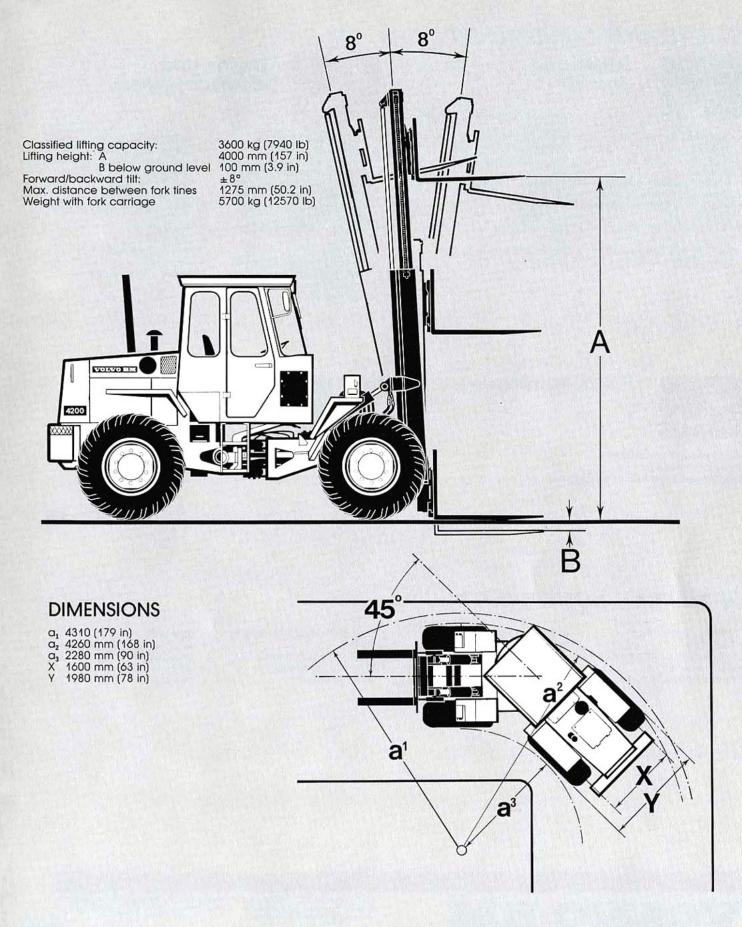
The specifications apply for a machine equipped with fork carriage and tyres 15.5–25/12.
