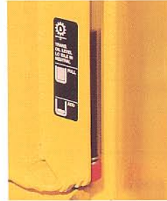
Visual sight gauge level checks provided for hydraulic and transmission fluid.
