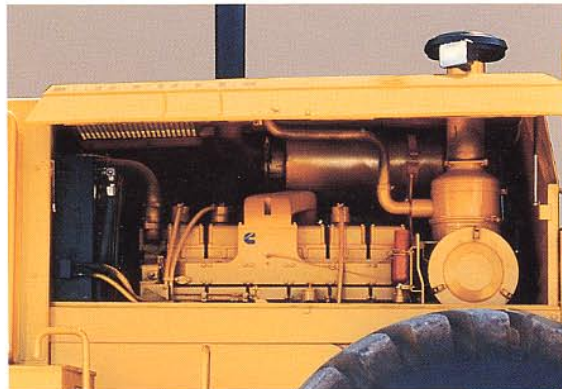
Hinged radiator grill and side panels for easy cleaning.
