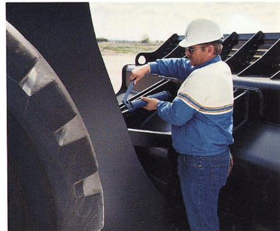
Grease fittings grouped so they can be lubed from four ground level locations.
