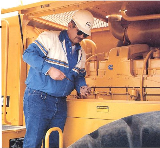
Engine oil level and fuel filters checked easily from service platform.
