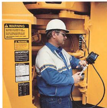
Quick-connect, remote pressure check ports save time and labor.
