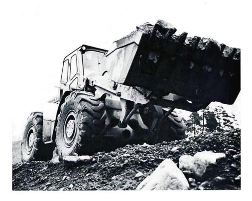
Excellent bucket angle enables maximum bucket loads to be transported without spilling.
