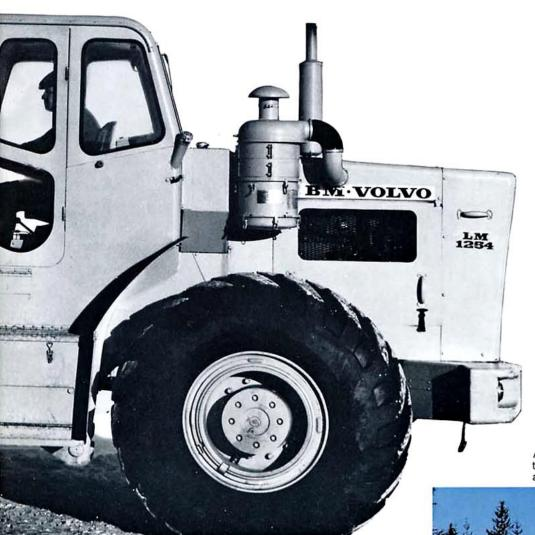
A total rear oscillation of 22° gives the loader exceptionally good traction and stability even on very rough ground.
