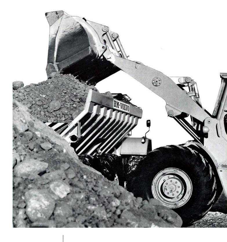
The LM 1254 has 4-wheel drive and good weight distribution. This ensures maximum utilization of machine weight and engine output to propel the vehicle, excellent ability to traverse loose ground and fine steering properties.
