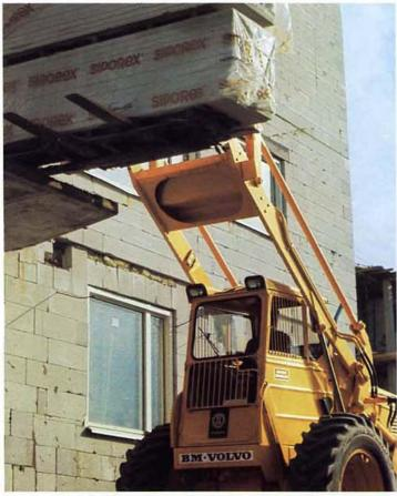
The outreach ahead of the tyres is long, enabling simple and rapid loading and unloading from truck platforms and railway wagons from one side. The parallel side-arm action in combination with high figures for lift and outreach make the loader ideal for handling palletized loads and timber. Consequently, the LM 621 is the obvious loader for construction sites, goods terminals, ports and for industrial applications.
