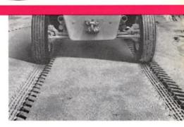
Turning circle radius is only 5 metres (16 ft.) and can be even further reduced by using steering brakes.
