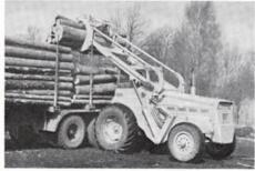
The LM 218 loader is built to toil untiringly under the most widely varying conditions. More than 50 different units are included in the implement range, which covers practically every conceivable application. Equipped with half-tracks and protective plates designed for forest driving, the LM 218 is a fine off-the-road worker in wooded terrain and over soft ground.
