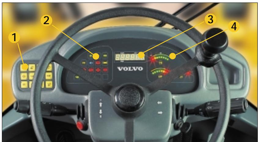
**1 Membrane key pad with symbols and integrated LEDs**
