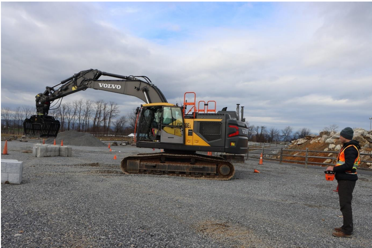
The EC250E excavator with Remote Control operation is on display at CONEXPO
