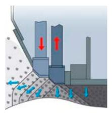
working width. Finished level tolerances are tighter controlled even with large variations in subbase conditions, thanks to the material being compacted twice before it leaves the screed. The vibration system subsequently ensures a smooth finish of the wearing course.
