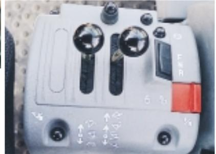
Pilot operated fingertip hydraulic levers provide easy control of the hydraulic functions. The adjustable hydraulic lever console also features a rocker switch for forward/reverse shifting and 1<sup>st</sup> gear kickdown button.
