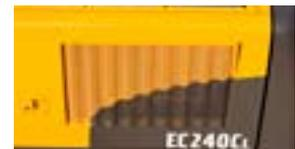
**Engine air-intake screen** prevents larger particles from entering the radiator compartment and maintains cooling performance for uptime and reliability.
