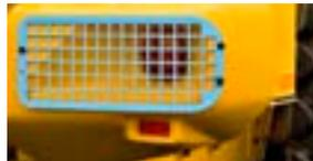
**Headlight guards and tail light guards** protect the headlights, work lights, tail lights and turn signals from debris that may break or damage the lenses.
