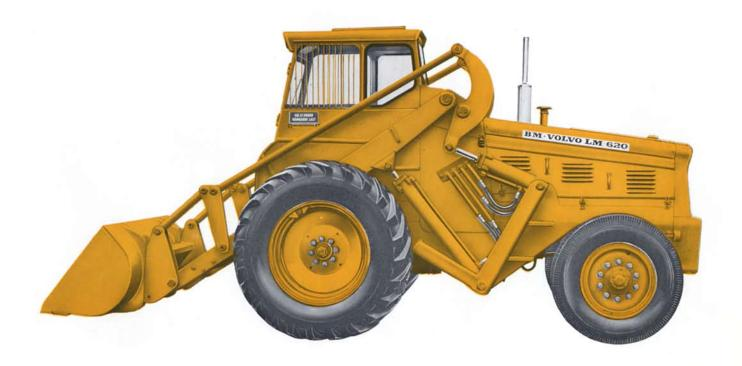
A 4-wheel drive loader for difficult ground conditions
