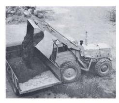
The BM-VOLVO implement attachment system permits the use of a very wide range of standard attachments. Because attachments can be changed so speedily, machines can be properly equipped for each job without unnecessary loss of time. The profitability of a loader is greatly dependent on the use of the right tool for the job and the line of
