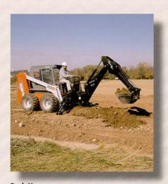
**Back Hoes**Heavy duty digging power for high production digging and trenching.
