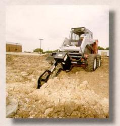
**Trenchers**Heavy duty attachments for installing sprinkler systems, underground utilities and silt fence.
