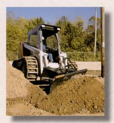
**Dozer Blade**Use for dozing and backfilling in tough grading conditions.
